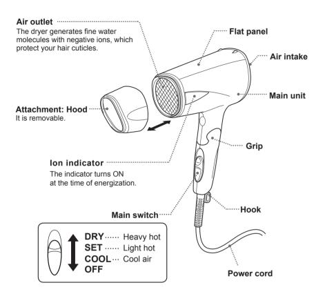
You can lay down the dryer on its flat panel when not using it.
