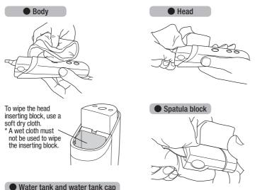
Discard the tank water. Then, after drying naturally, reinstall the tank on the body.
